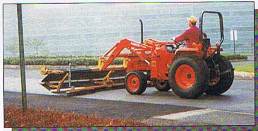
Installation equipment is available to mount as attachments on tractors (right), the back of the oil spreading trucks, tractor end loader arms, and on buckets (top right).
