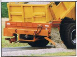
The Concord Berming Machine conveyor is a completely reversible. safe and quick way to do various jobs such as road berming, repairing washouts, asphalt patching, curb building and french filling. Add the spinner attachment for spreading ice control materials making your machine versatile year round! Use your Concord Berming Machine wherever you need to move material from your dump body to a desired location without spending unnecessary time and labor.
