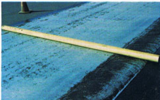
Figure 1: Heat shrinkage is quickly and easily measured with the use of an empty core.
