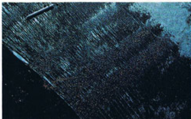
Figure D: If fabric is installed too close to the hot oil truck, excessive shrinkage and melting damage occurs.
