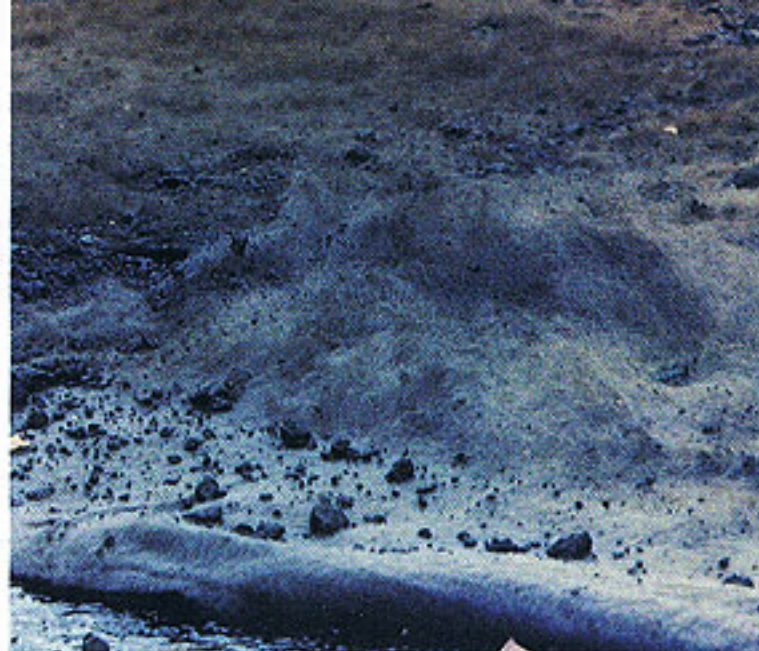
Figure A: Delamination or fuzzing commonly occurs in non-heat bonded paving fabrics.
